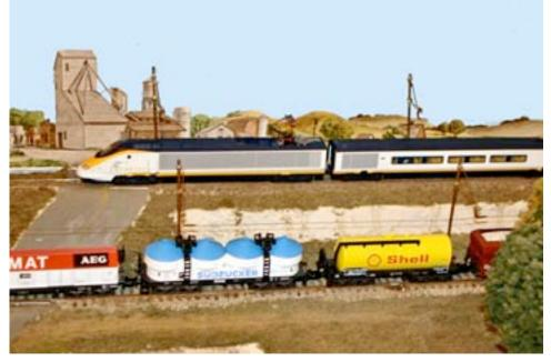
*N*-Cat using "live" catenary. Note the single pantograph on the rear of the power unit.
