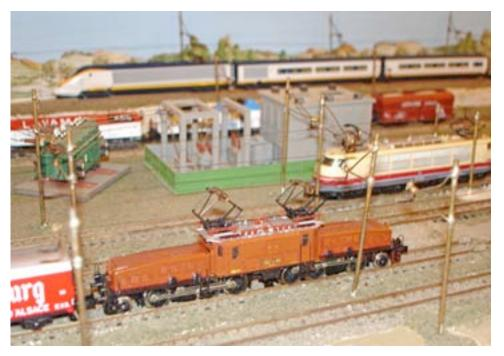
A busy yard area using "live" catenary power. Note the pantographs used to get power for the consists. NTRAK Page 9
