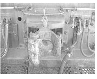
is a reference to this coupler pin! If the engineer and brakeman work together so that the coupling is accomplished gently, the couplers join together so that the pin drops quietly enough to hear it go "clink". This phrase is one of many that originated on the railroad.
