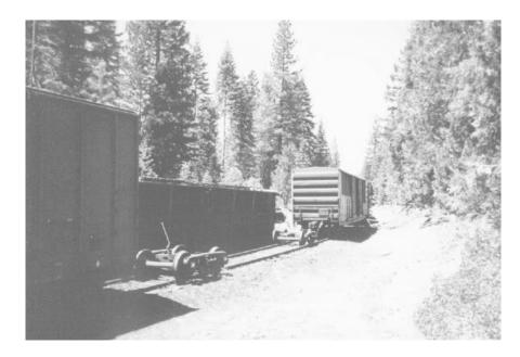
Bear Flat, CA, 5/2003. This is one of several boxcars stored on the branch that are laying completely on their sides as a result of the uneven snow melt off of the car roofs. The great winter of 1992-1993 tipped over more than 20 boxcars stored on the Pondosa branch, as well as several more stored on the Bartle siding.
