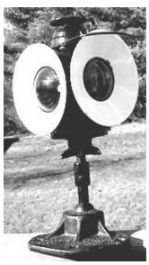
This is actually a railroad lamp, not a lantern. Lanterns and lamps differ from each other in both function and design. Lanterns were typically carried in the hand of railroad worker, while lamps were mounted or hung in a location and were only taken down to be cleaned.
