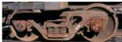
Fig. 14 100-TON RIDE CONTROL TRUCK. The 100-ton version of the ASF Ride Control truck has three visible springs. Note the differing styles of bearing and caps on each axle.
