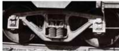
Fig. 8 BARBER S-2 TRUCK. The Barber Stabilized truck design was among the most commonly used types of freight car trucks through the end of the solid-bearing-truck era.
