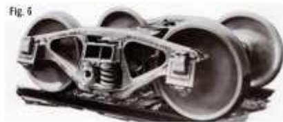
Fig. 5 AAR U-SECTION TRUCK. Trucks with U-shaped sideframe cross sections were built by several companies. The modified sideframe was stronger than the older T-section truck design.
