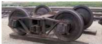
Fig. 2 ARCHBAR TRUCK. Archbar trucks are made of numerous pieces of pressed steel and bar components bolted together. The trucks worked well, but the bolts tended to loosen over time. They were banned from interchange service starting December 31, 1939.
