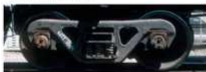
Fig. 15 100-TON BARBER S-2 TRUCK. Modern freight car trucks are similar in appearance, but if you look carefully, this S-2 truck has subtle differences in shape compared to the Ride Control truck.
