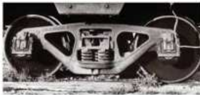
Fig. 9 ASF A-3 RIDE CONTROL TRUCK. This truck became the most popular truck of the post-World War II era.
