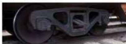
Fig. 16 BARBER-BETTENDORF CABOOSE TRUCK. The most popular modern-era caboose truck was the roller-bearing-equipped version of the venerable Barber-Bettendorf truck.
