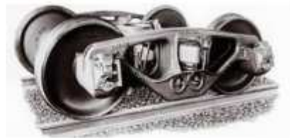
Fig. 10 NATIONAL B-1 TRUCK. This truck can be distinguished from others by its unique spring package and side-frame design.
