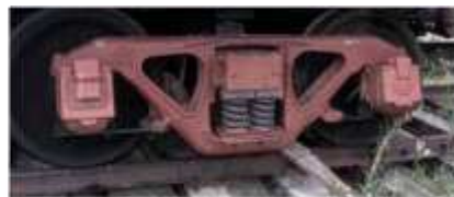
Fig. 3 ANDREWS TRUCK. These trucks have cast steel sideframes with journal boxes bolted in place. The steel retaining straps extending from the base of the journal box to the sideframe identify this as an Andrews truck. This one was built by the Bettendorf Co.
