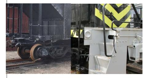
Poling pockets were used as an alternate way of moving cars without coupling the engine to the car. A end of a wooden pole would be placed in one pocket of the car and the other end in a pocket of the engine (which was on an adjacent track) to push the car into position. This practice was discontinued by most railroads in the 1960's.
